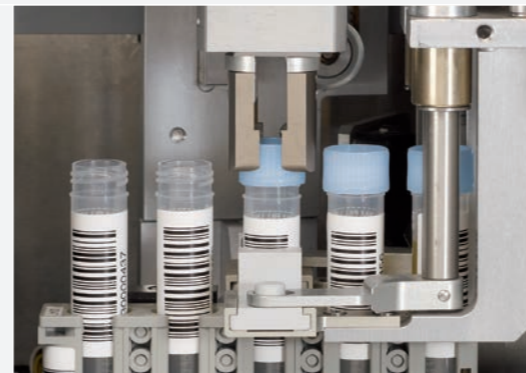
Recapping: Screw cap
